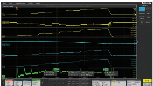
▲ Fig. 14 The output current is stepped, and the input power and output power are monitored and divided to provide the efficiency data in a 1.5 ms acquisition without any cooling.
