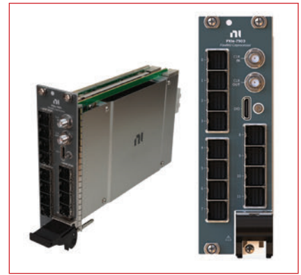
▲ Fig. 8 NI PXIe-7903 Flex-RIO HSS module. Source: Based on Xilinx Virtex UltraScale+ VU11P FPGA with 48 multi-gigabit transceivers.
