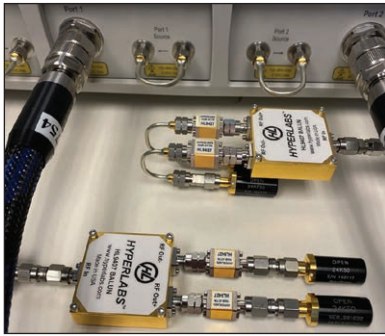
▲ Fig. 5 Open reflection calibration of port 1.
