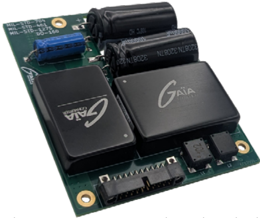
Figure 5: The 3.5"×3.30" 40 W power supply complies with Mil-STD-461, Mil-STD-704 and DO-160 with hold-up function thanks to the FLHG-60-MN integrated front end.
